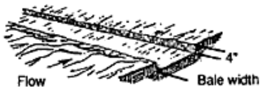
Figure 3: Constructing a straw bale barrier to slow runoff and prevent erosion.
